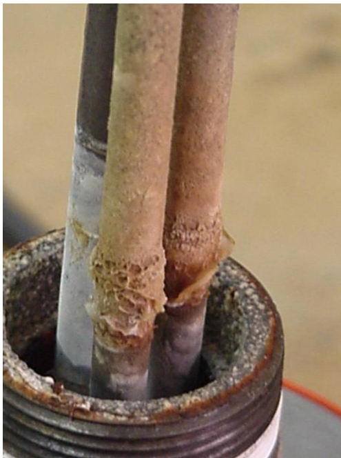
Figure 14: Base of experimental heating element with sufficient scale removed after 4 days of electrostatic treatment.
