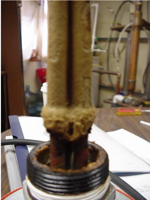
Figure 13: Base of experimental heating element with sufficient scale formed after 5 days without electrostatic treatment.
