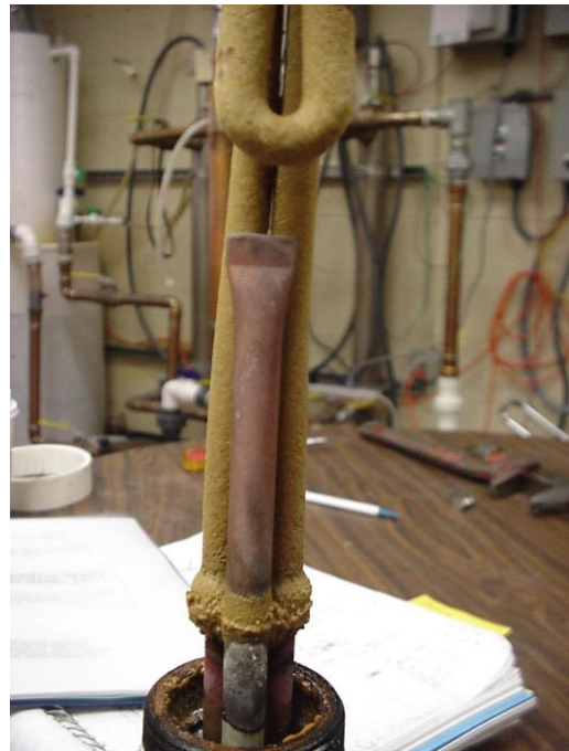
Figure 12: Experimental heating element with sufficient scale formed after 5 days without electrostatic treatment.
